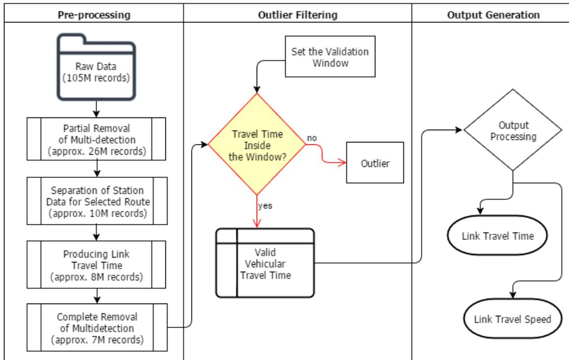
**FIGURE 2 Data processing procedures.**
